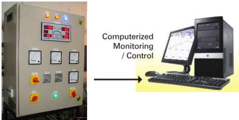
Note: Libratherm offers ready to use control panel for single phase or 3 phase wax burnout furnace built using solid state relays or thyristor based power regulators (3 KW to 100KW)
